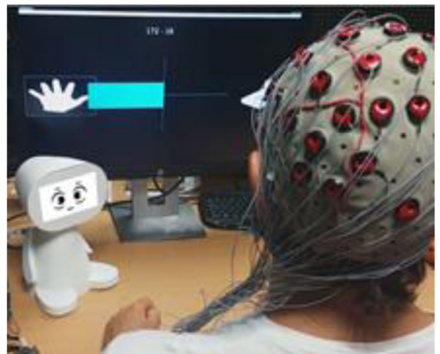
Fig. 3. Brain–computer interface training during which PEANUT (on the left) provides user with social presence and emotional support adapted to his performance and progression [62].
